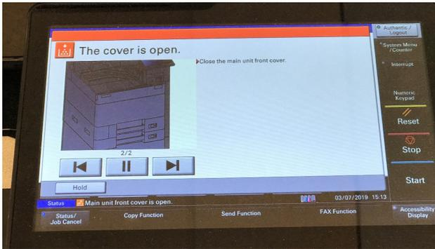
Users are also presented with an animated video to help clear misfeeds; users can let the video play or scroll through step by step using the arrows at the control panel.
